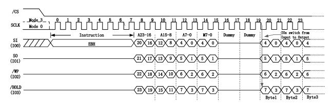
**Figure 7.2.6a.** Fast Read Quad I/O Instruction (Initial instruction or previous M5-4  $\neq$  10)
