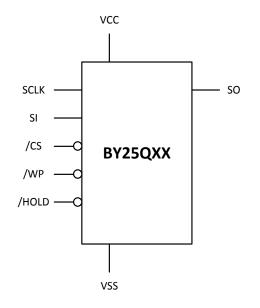
Figure 2. Pin Configuration SOP8/TSSOP8
