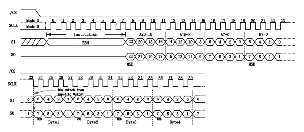
Figure 7.2.5a. Fast Read Dual I/O Instruction (Initial instruction or previous M5-4 $\neq$ 10)
